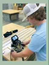
Mr. Luettel's Cabinet I woodworking students are testing out the new Shaper Origin. It's a hand-held CNC machine. Students work on using offsets, design software, and tolerances needed in manufacturing and construction. This student pictured is cutting out 14 inch circles for his project.
